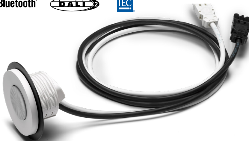
P40 detector series 230 V with SnapFit mounting and medium detection range 12-13 m
