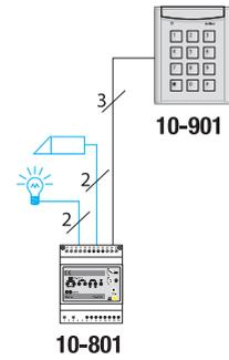
This code keyboard for surface mounting is suitable for indoor and outdoor applications. It is made of aluminium and is illuminated with 4 blue LEDs. You can program the code keyboard with a maximum of 10 different users codes. Different functions can be assigned to each code, e.g., door opener bus power supply, external relay contact etc.
